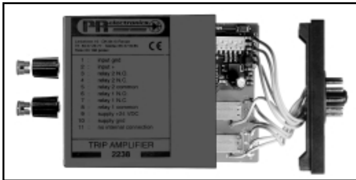
Picture 3: Removal of PCB for adjustment of dip switches and replacement of jumpers.
