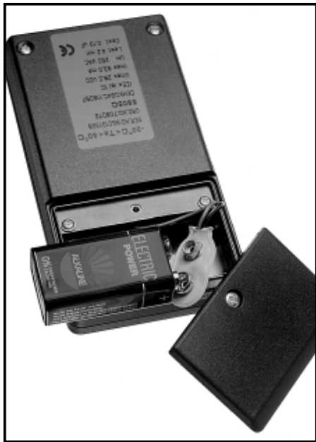
Picture 1: Replacement of battery.
